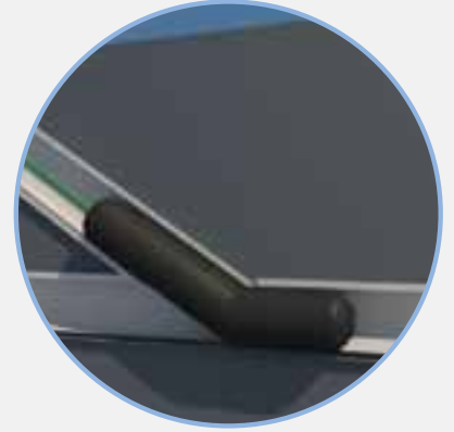
IN THE SECOND PHASE, THE REMAINING PART OF THE PLUG IS INFLATED TO COMPLETELY STOP THE FLOW
